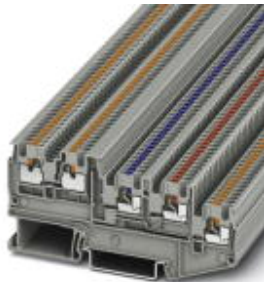
Sensor/actuator terminal block, Connection method: Push-in connection, Cross section: 0.14 mm 2 - 1.5 mm 2 , AWG: 26 - 14, Width: 3.5 mm, Color: gray, Mounting type: NS 35/7,5, NS 35/15
