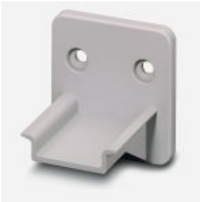
Plastic mounting bracket, with NS 35/7.5 DIN rail, to snap onto modular terminal blocks with a universal foot, profile length: 19 mm
