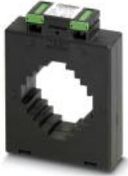
Window-type current transformer, 1,250 A AC primary current; 5 A AC secondary current; accuracy class 1; 10 VA rated power
