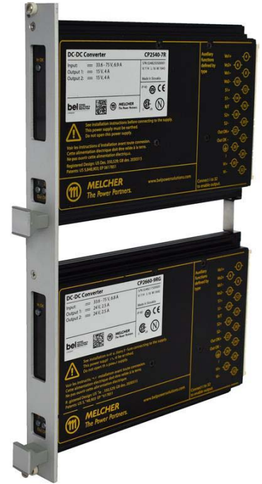
Front panel kit G05-6HE-Q01 (HZZ00838) accommodating two HP units for a 19" DIN-rack with 6 U, 5 TE.
