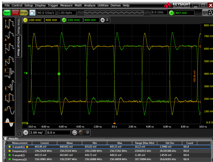
Figure 5-1. LVPECL 3.3 V, 156.25 MHz Clock Measured with DC Coupling, 50-Ω Scope Termination
