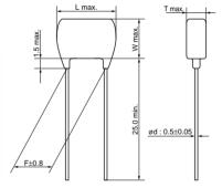
· Lead Wire: Solder Coated Copper Wire or Solder Coated CP Wire
