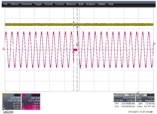
CH1:Vo (10 V/div) CH2:Vin (200 V/div) Figure 10: AC drop out 12 mS at 230 VAC (50 mS/div)
