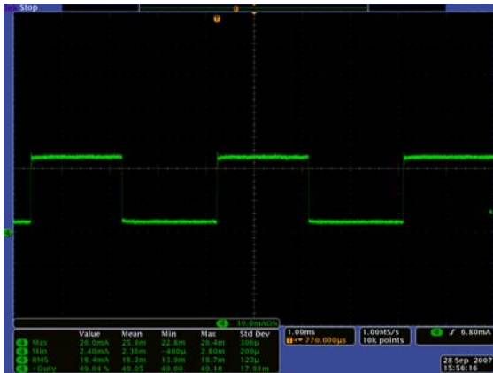
FIGURE 16. I LED AT 50% PWM DIMMING
