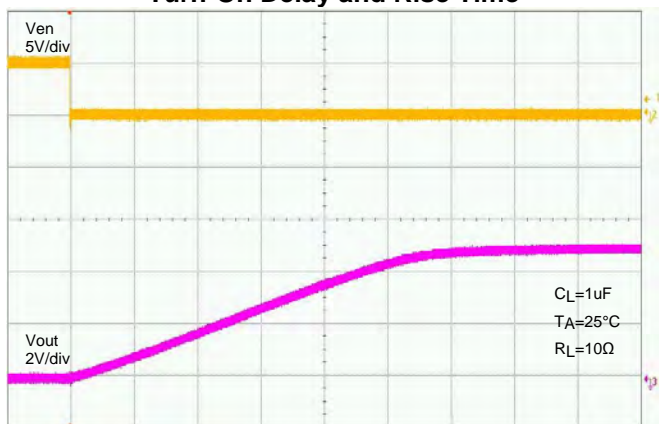
Turn-On Delay and Rise Time
