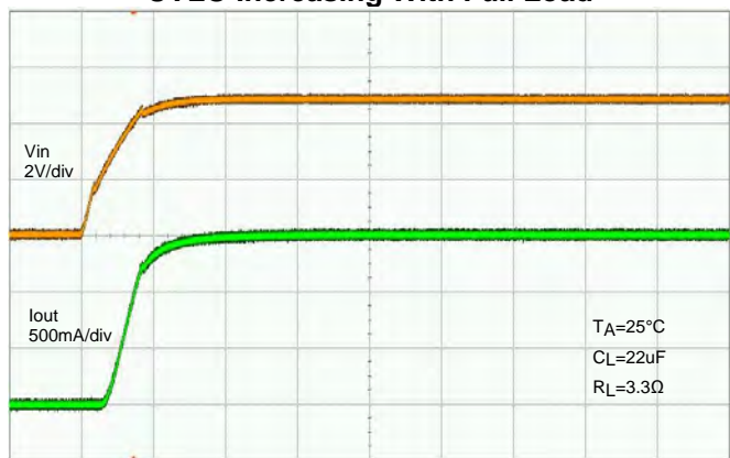
UVLO Increasing With Full Load
