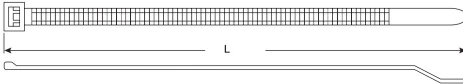
One piece, self locking cable ties are molded of tough, corrosion resistant and electrically insulating nylon 6/6. Smooth, rounded design prevents damage to insulation and components. Wire tie features a unique, double bend, tapered tip for fast, easy insertion and assembly. Ties can be installed by hand or with available installation tools. Ultra-violet stabilized black nylon ties are available upon request.
