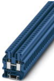
Mini feed-through terminal block, Connection method: Screw connection, Cross section: 0.2 mm 2 - 6 mm 2 , AWG: 24 - 10, Width: 6.2 mm, Color: blue, Mounting type: NS 15
