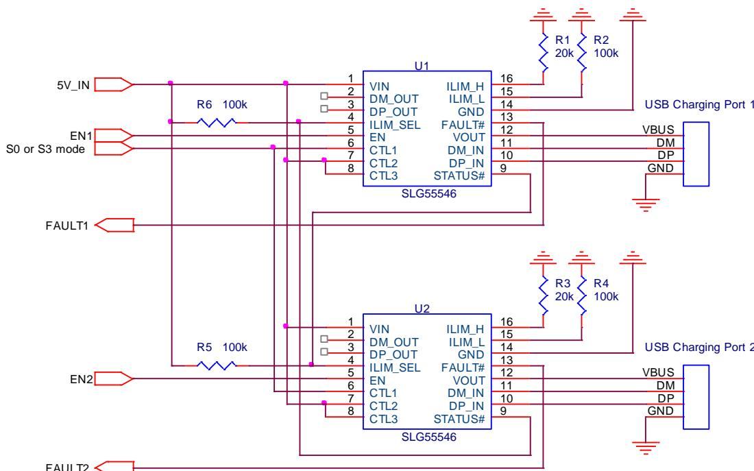
Figure 1. Implementing PPM with two independent charging ports
