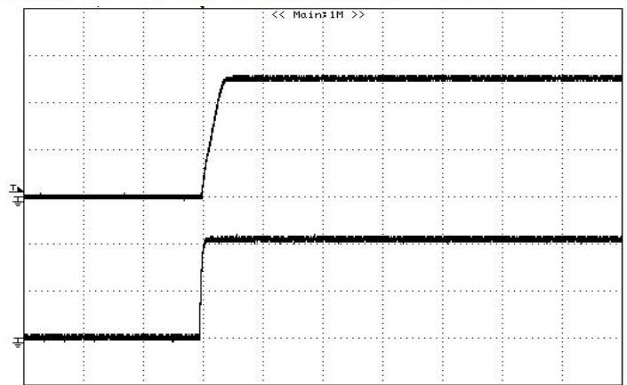
**Figure 20:** Turn on delay time at Remote On/Off, 5V/3A out
