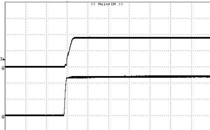
**Figure 15:** Turn on delay time at 12Vin, 0.9V/3A out
