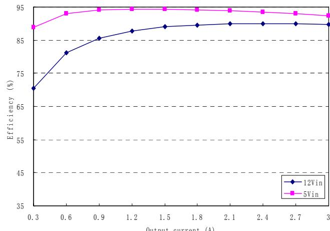
**Figure 5:** Converter efficiency vs. output current
