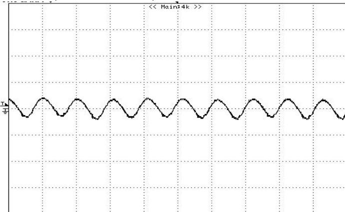
**Figure 9:** Output ripple & noise at 12Vin, 1.8V/3A out
