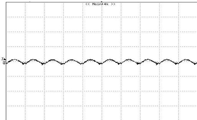
**Figure 7:** Output ripple & noise at 12Vin, 0.59V/3A out
