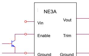
**Figure 26:** Enable Input drive circuit for NE series
