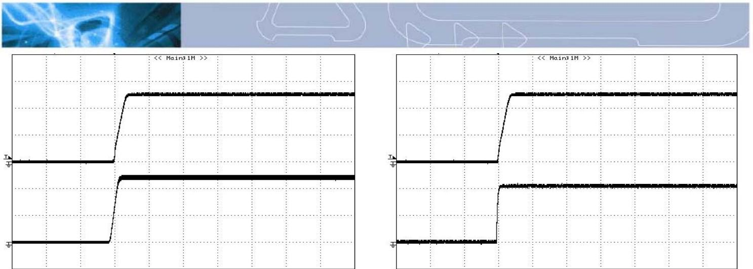
**Figure 19:** Turn on delay time at 12Vin, 5V/3A out
