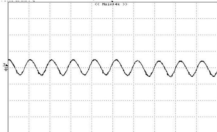
**Figure 10:** Output ripple & noise at 12Vin, 2.5V/3A out
