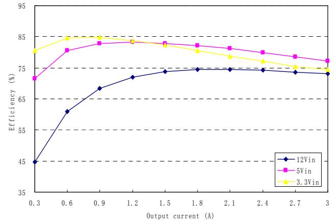
**Figure 2:** Converter efficiency vs. output current
