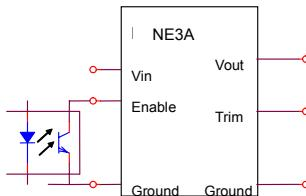
**Figure 27:** Enable input drive circuit example with isolation.
