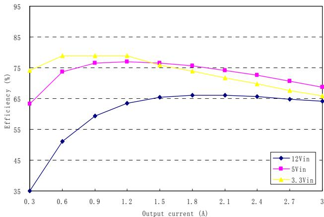
**Figure 1:** Converter efficiency vs. output current
