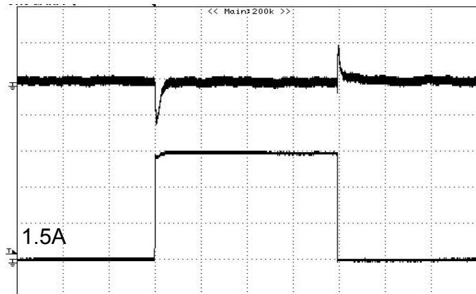
**Figure 23:** Typical transient response to step load change at
