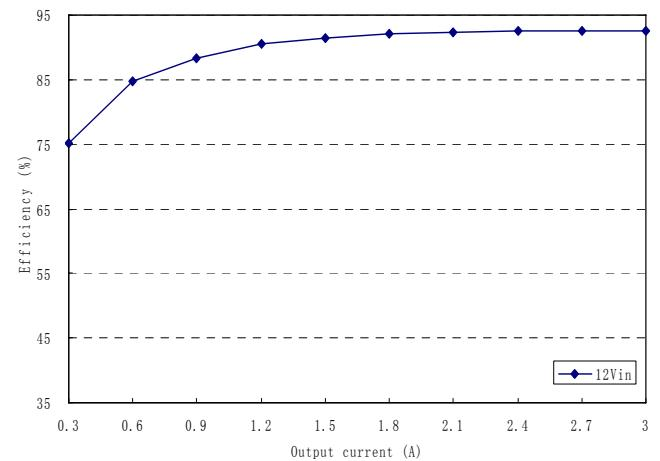
**Figure 6:** Converter efficiency vs. output current
