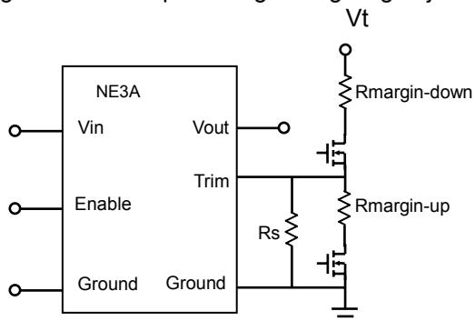
Figure 31: Circuit configuration for output voltage margining
