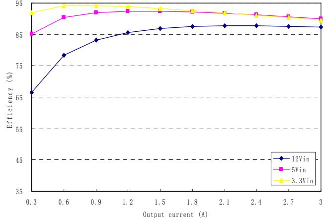
**Figure 4:** Converter efficiency vs. output current
