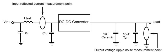
$C_s = 270\mu F \times 1$ ,  $L_{\text{test}} = 2\mu H$ ,  $C_{\text{in}} = 270\mu F \times 1$
