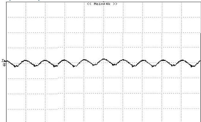
**Figure 8:** Output ripple & noise at 12Vin, 0.9V/3A out
