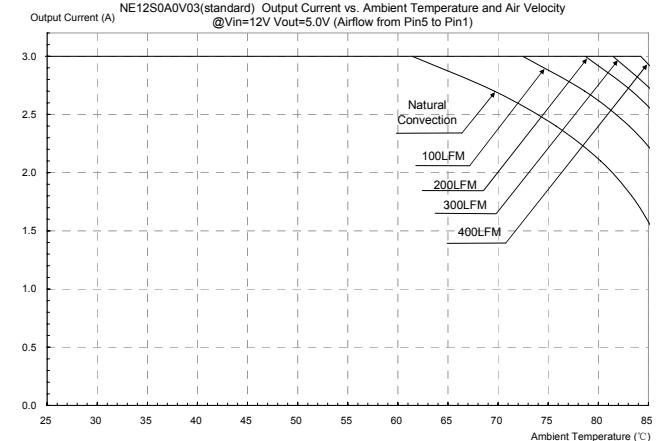
**Figure 41:** Output current vs. ambient temperature and air velocity@ Vin =12V, Vout=5.0V (Airflow from Pin5 to Pin1)
