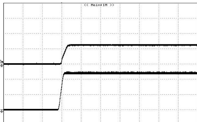
**Figure 17:** Turn on delay time at 12Vin, 2.5V/3A out
