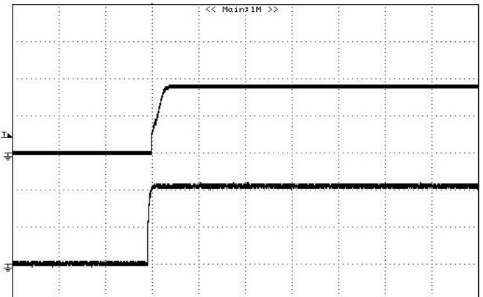
**Figure 16:** Turn on delay time at Remote On/Off, 0.9V/3A out
