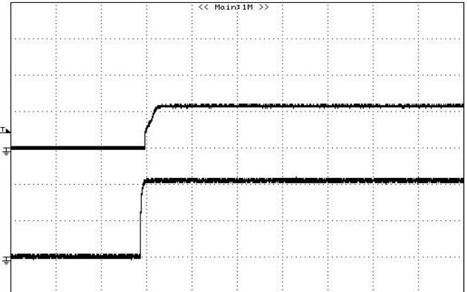
**Figure 14:** Turn on delay time Remote On/Off, 0.59V/3A out
