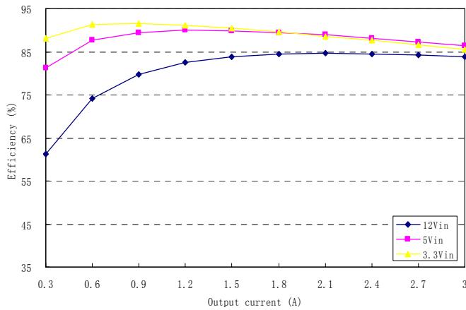
**Figure 3:** Converter efficiency vs. output current
