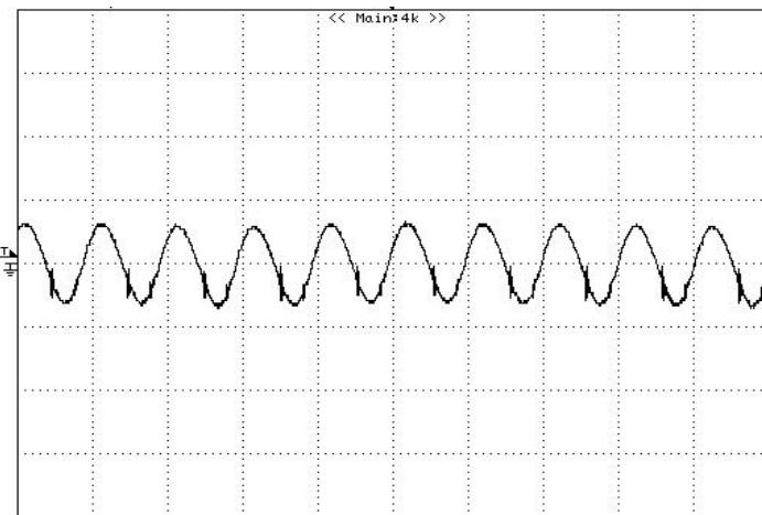
**Figure 11:** Output ripple & noise at 12Vin, 3.3V/3A out
