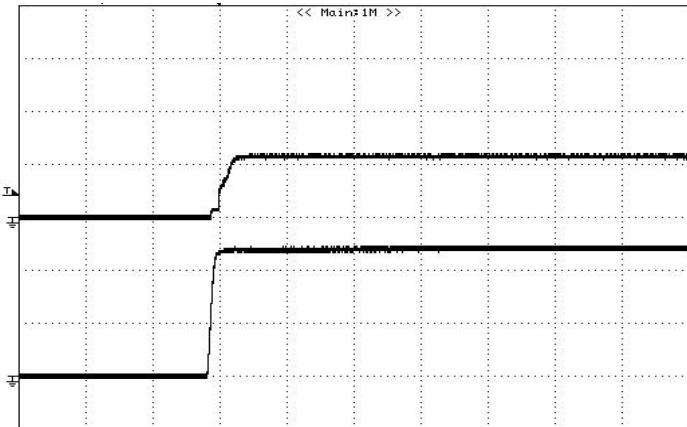
**Figure 13:** Turn on delay time at 12Vin, 0.59V/3A out
