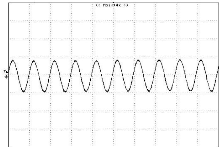
**Figure 12:** Output ripple & noise at 12Vin, 5.0V/3A out
