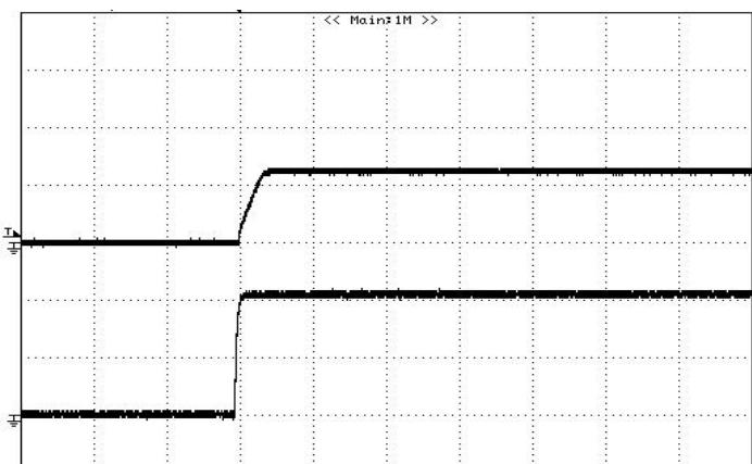
**Figure 18:** Turn on delay time at Remote On/Off, 2.5V/3A out
