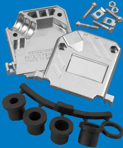
Amphenol's plated plastic backshell accommodates most standard and high-density D-Subminiature connectors and is appropriate for cable assemblies requiring compliance to FCC 20780. This version is highly durable and provides EMI/RFI protection. The rubber grommet compression insert forces the cable's shielding against the inside of the cable exit area, assuring shielding. The 45° cable exit helps save space behind equipment.
