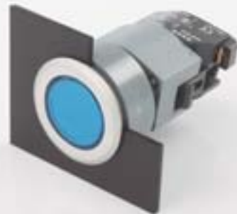
Indicator, flush mount, aluminum bezel, 30.5mm mounting
