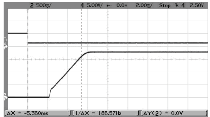
On/Off Enable Startup ( V_{IN}=5V , V_{OUT}=1.8V , I_{OUT}=6A , C_{LOAD}=0 ) Trace 4=Enable, Trace2=Vout
