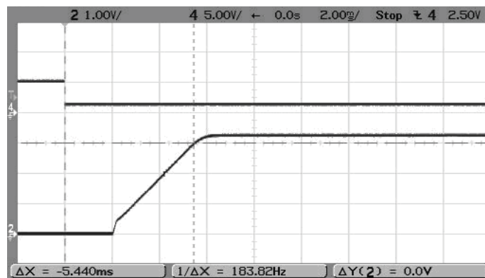
On/Off Enable Startup (V in =5V, V out =3.3V, I out =6A, C load =0) Trace 4=Enable, Trace2=V out
