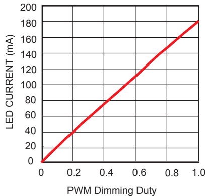
LED Current vs. PWM Dimming Duty
