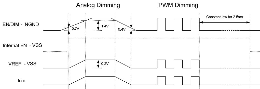
**Figure 2—Internal EN Shut-down Delay Function Waveform Diagram**
