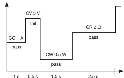
The 8600 Series can execute multiple test sequences in automatic test mode. Up to 100 different sequences can be linked to run steps of various operating modes and loading conditions. Each sequence can also be programmed with upper and lower limit Pass/Fail criteria. When applied in production testing, you can easily judge whether the test parameters of your devices are within the specification limits and adjust your process according to the Pass/Fail verdict.
