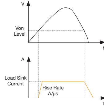
Control the input turn on state for the DC electronic load by configuring the Von latch function. This can be used to start and stop discharging of a battery or other power source at a specified voltage level.
