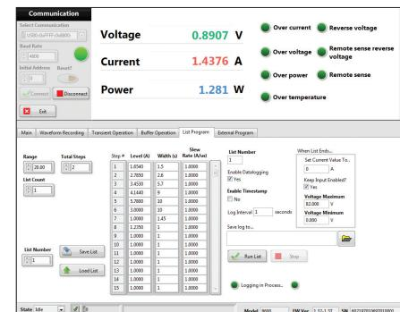
PC software is provided for front panel emulation, generating and executing test sequences, or logging measurement data without the need to write source code. Additionally, this application software integrates with NI Data Dashboard for LabVIEW apps, which allows users to create a custom dashboard on a tablet computer or smartphone to remotely monitor 8600 Series DC loads via this PC software.
