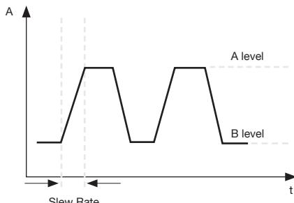
Transient operation enables the module to periodically switch between two load levels. A power supply's regulation and transient characteristic can be evaluated by monitoring the supply's output voltage under varying combinations of load levels, frequency, duty cycle, and slew rate. Transient operation can simulate these conditions.
