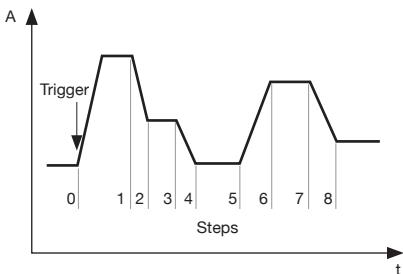
List mode lets you generate more complex sequences of input changes with several different levels. Up to 7 groups of list files can be saved. Each list can contain up to 84 steps with a minimum width time of 20 µs per step.
