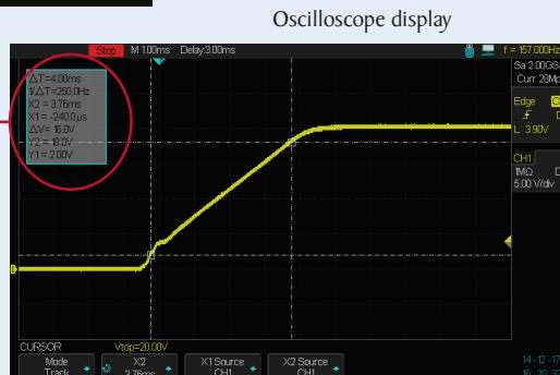
The 8600 Series can measure the rise or fall time from a specified start and stop voltage level of the measured input without the need for an oscilloscope. This function can also be used as an internal timer to count how long the input has been enabled.
