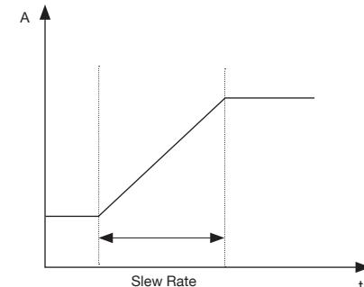
In CC mode, users can control the rate or slope of the change in current in a transient response test. Set the slew rate to as slow as 0.001 A/ms or as fast as 2.5 A/μs depending on the model and selected current range.
