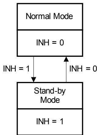
**Figure 5 Mode State Diagram**
