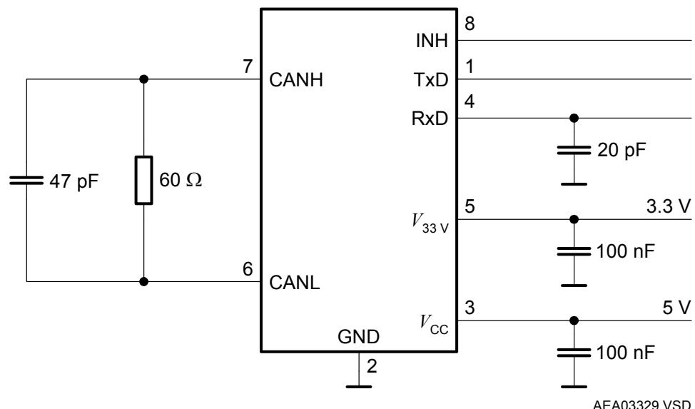
Figure 3 Test Circuit for Dynamic Characteristics
