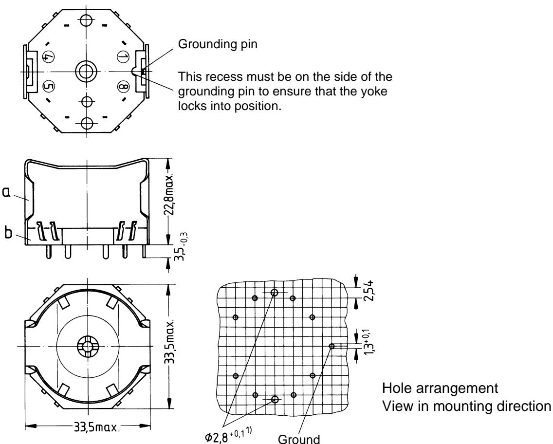
1) The 2.8 mm hole is only necessary for additional fixing with M 2.5 screw.
