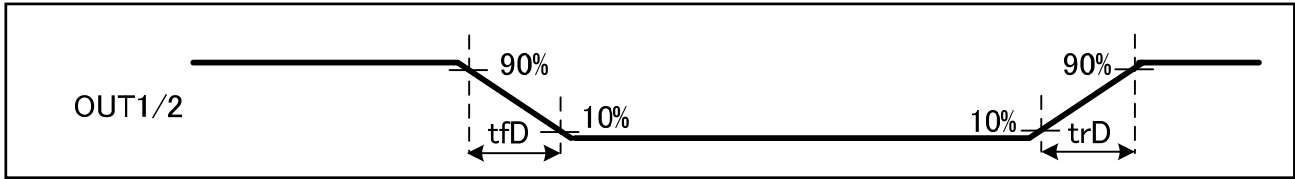
Figure 10.9-1 Slew rate of driver output (SR)
