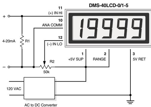
**Figure 7. 4-to-20mA Current Loop Operation (5V-Powered Models)**
