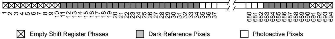
Figure 13. Line Timing Diagram – Single Register Output
