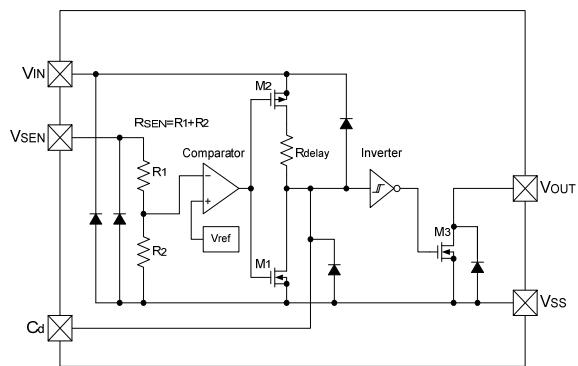
\*The delay capacitance pin (Cd) is not connected to the circuit in the block diagram of XC6118NxxD (semi-custom).
