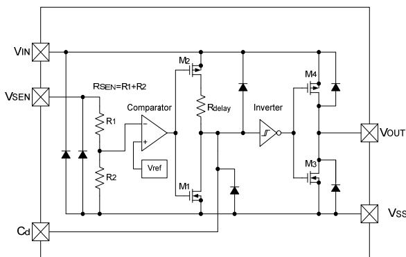
\*The delay capacitance pin (Cd) is not connected to the circuit in the block diagram of XC6118CxxD (semi-custom).
