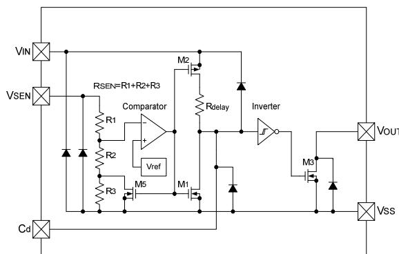
\*The delay capacitance pin (Cd) is not connected to the circuit in the block diagram of XC6118NxxC (semi-custom).
