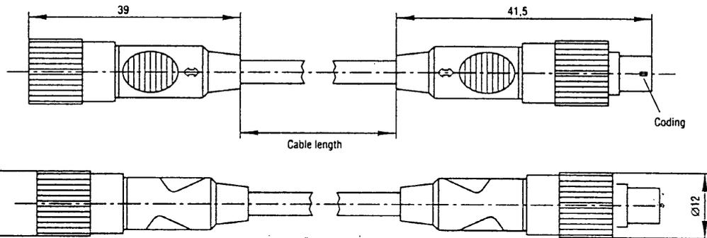
Cable with overmoulded connector
