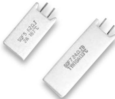
As the Thermal fuses are incorporated, these cement filled resistors respond quickly to overloading as well as to external overheating. The SQF series also provides outstanding features against surges, and are therefore suitable for the preventing of inrush current for switching regulators. Obvious economic advantages can be achieved by not having to specify a separate thermal fuse.
