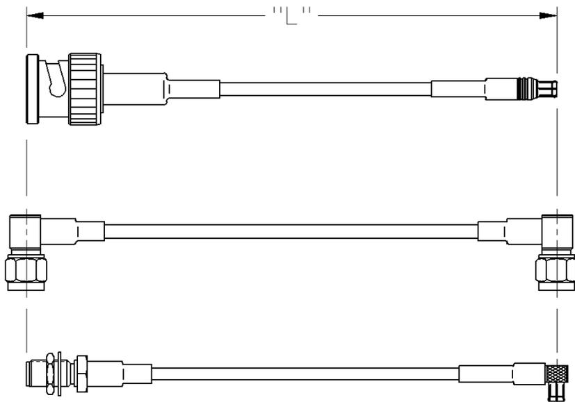
Johnson Components' cable length applies to the end of straight connectors. The length is applied to the vertical centroid of right angle connectors. The last three digits of the part number reflect the length of the cable in inches.
