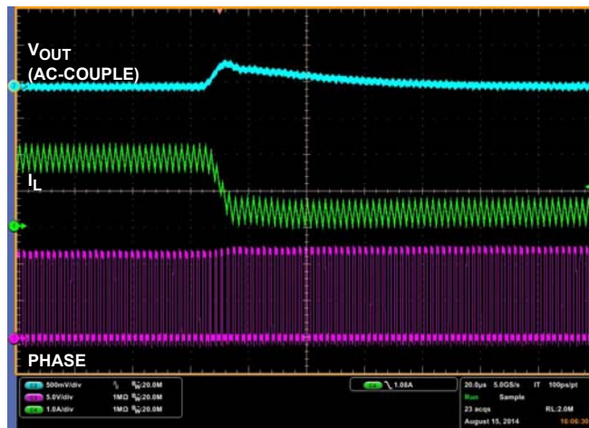
FIGURE 12. LOAD TRANSIENT RESPONSE
