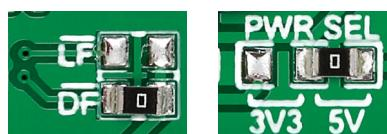
Counter click has two SMD jumpers [zero ohm resistor]. One lets you switch between a 3.3V or a 5V power supply. The other is for setting the interrupt as LFLAG [open drain latched output] or DFLAG [push-pull output].
