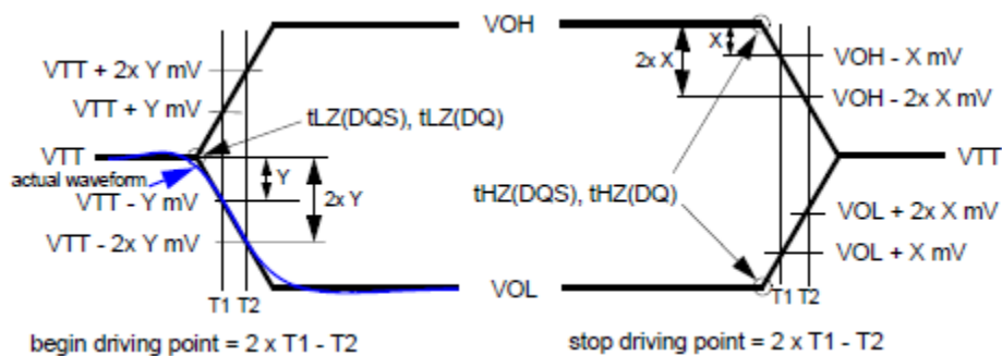
Figure 11.1 — HSUL_12 Driver Output Reference Load for Timing and Slew Rate
