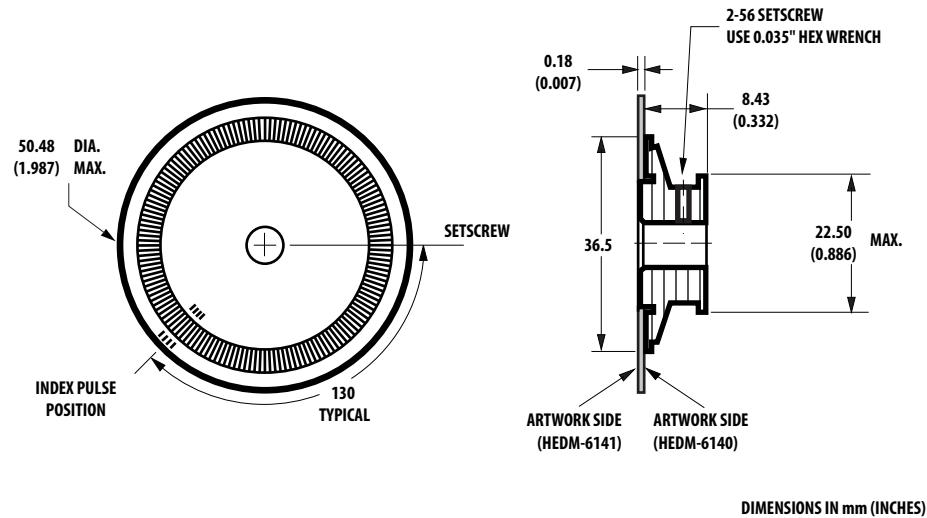
Figure 12. HEDM-6140 Codewheel/HEDM-6141 Codewheel.
