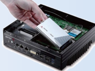
2. One screw removable storage bracket
