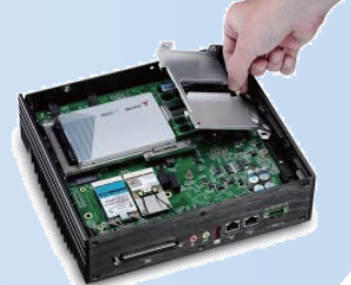
3. Flexible memory expansion slots
