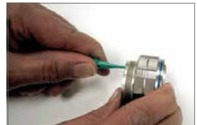
Plastic tool with contact in proper position.
