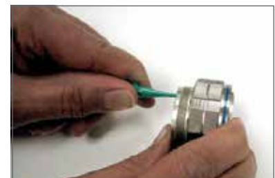
Plastic tool with contact in proper position.
