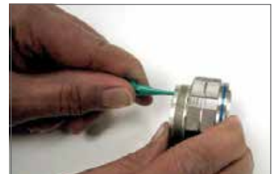
Plastic tool with contact in proper position.
