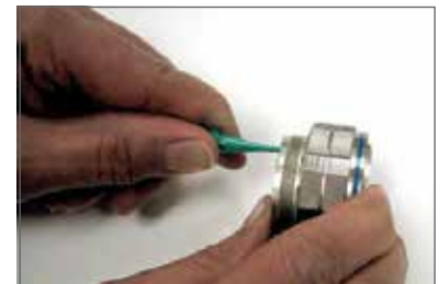
Plastic tool with contact in proper position.
