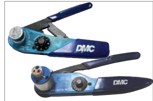
Examples of M22520 Series Crimping Tools:
