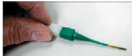
Plastic tool with contact in proper position.
