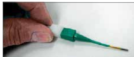
Plastic tool with contact in proper position.
