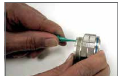
Plastic tool with contact in proper position.
