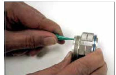
Plastic tool with contact in proper position.
