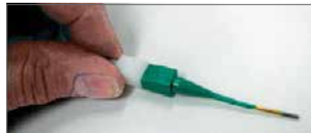
Plastic tool with contact in proper position.
