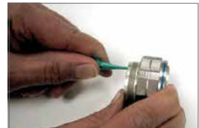
Plastic tool with contact in proper position.
