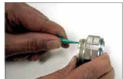
Plastic tool with contact in proper position.
