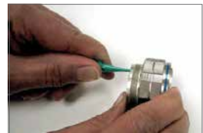
Plastic tool with contact in proper position.
