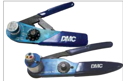
Examples of M22520 Series Crimping Tools:
