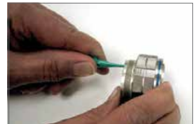
Plastic tool with contact in proper position.
