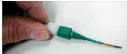
Plastic tool with contact in proper position.
